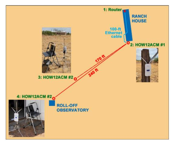
available in the north end of the Ranch House located on the Cat-Star Sky Ranch property. This service is provided by CapRock Telephone (https://www.caprock-spur.com/) via their regional fiber optic system. A router at this point provides local WiFi service for the Ranch House and Ethernet connections for other devices.
